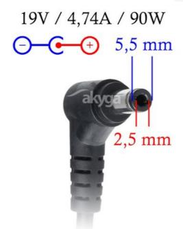
Akyga AK-ND-10 is a 90W laptop power supply dedicated to Acer, ASUS, Aristo, Benq, IBM/Lenovo, HP/Compaq, and Toshiba laptops. The power supply is compatible with all models powered by 19V/4.74A and with a 5.5\*2.5 mm connector. The complete set of protections OVP, OTP, OPP, SCP, and OCP, along with soft start functionality, ensures safe and stable operation of the power supply and powered devices.
