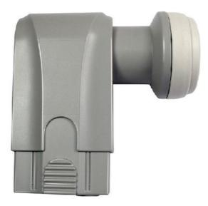
The Unicable II dLNB dCSS converter, or Digital Channel Stacking System, allows you to provide up to 24 or 32 transponders with different polarity via a single wire, which allows you to decode multiple programs in several tuners at the same time. UNICABLE system standards: EN50494, UNICABLE I, 8 channels EN50607, UNICABLE II, 24 channels
