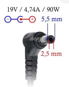
Akyga AK-ND-10 is a 90W laptop power supply dedicated to Acer, ASUS, Aristo, Benq, IBM/Lenovo, HP/Compaq, and Toshiba laptops. The power supply is compatible with all models powered by 19V/4.74A and with a 5.5\*2.5 mm connector. The complete set of protections OVP, OTP, OPP, SCP, and OCP, along with soft start functionality, ensures safe and stable operation of the power supply and powered devices.
