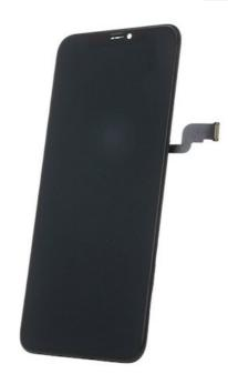
Service Pack + is a refurbished original display. All components are original except for the front protective glass, which is a high-quality replacement of the screen includes all necessary elements for installation in the smartphone: - camera holder, - sensor holder, - speaker cover, - foam pads on ribbons. The foam pads prevent excessive bending of the ribbons and disconnection during phone use.
