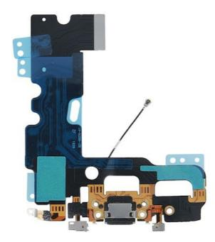
The presented product is a high-quality flex tape with a charging connector, a lower antenna and a microphone. The tape is easy to install and a not require soldering.
