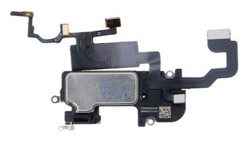
The presented product is a high-quality speaker tape with a set of sensors and a speaker. The tape is easy to install and does not require soldering
